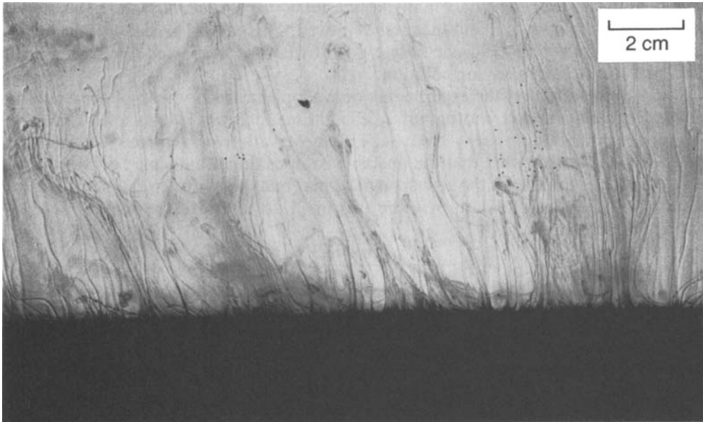
FIGURE 4. Photograph of a wax floor that is melting owing to being overlain by a hot dense aqueous solution of \text{NaNO}_3 .
